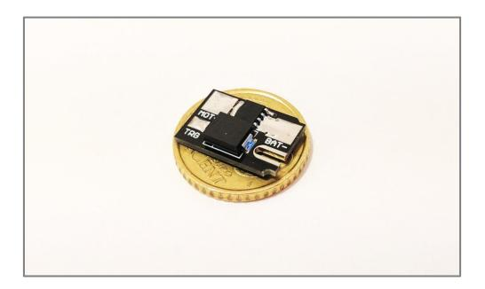
MicroFET is a basic MOSFET unit for an AEG rifle that redirects the current flow from the mechanical trigger to the unit and in effect lengthens the life of the gun, improves the response time, increases the rate-of-fire and improves the efficiency.
