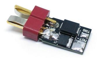
NOTE: Be very careful when soldering to not overheat the unit. Keep the soldering iron on the contact for not more than a few seconds. Immediately after soldering, you can cool down the unit by blowing on it.
